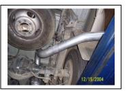
INSTALL EXIT PIPE #F ONTO PIPE #E. USE CLAMP #I TO SECURE TOGETHER. DO NOT TIGHTEN. INSERT WELDED HANGERS INTO RUBBER GROMMETS. ROLL EXIT PIPE TO GET THE BEST FIT FOR YOUR VEHICLE.
