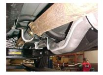
INSTALL DOWN PIPE #B ONTO DOWN PIPE #A. USING GASKET # H AND BOLT KIT # G. INSERT WELDED HANGERS INTO RUBBER GROMMETS. DO NOT TIGHTEN.
