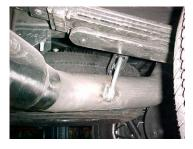
INSTALL THE OVERAXLE TAIL PIPE #D INTO THE MUFFLER 11/2"-2", SECURE TO MUFFLER USING CLAMP #F. INSERT WELDED HANGERS INTO RUBBER GROMMETS. DO NOT TIGHTEN.
