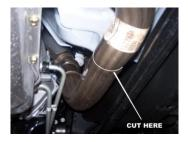
Cut factory down pipe just before converter (see picture). Then unclamp it from the turbo and remove. Save clamp it will be reused.
