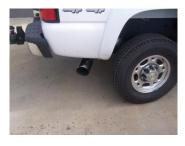
Install stainless steel tip. Clamp down. When you have everything in place, firmly tighten all bolts and clamps down securely. To clean stainless steel tip, use stainless steel cleaner and a Scotch Brite pad.
