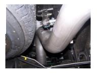
Install the overaxle tail pipe #D into the muffler 1½-2". Secure to muffler using clamp #F. DO NOT TIGHTEN.
