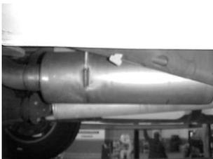
Install muffler #D onto intermediate pipe #B 1-1/2"-2". Use clamp #H to secure to down-pipe. Do not tighten. Inlet of muffler will have louvers facing forward.
