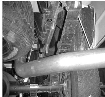
Install the exit pipe # F on to the tailpipe. Insert welded hanger into rubber grommet. Secure together with clamp # H. Do not tighten. Roll the exit pipe and tailpipe until it is at the correct angle for your truck with proper clearances.
