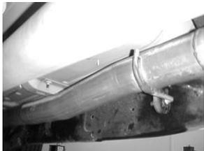
Install down-pipe # A on to your turbo using your factory clamp. Do not tighten. Insert welded hanger into rubber grommet.
