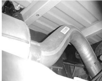
Install the over axle tailpipe # E into the muffler 1-1/2" to 2". Secure to the muffler using clamp # H. Do not tighten.
