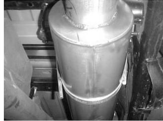
Install band clamp #I onto muffler with hanger rods facing forward and insert hangers into rubber grommet. Do not tighten.
