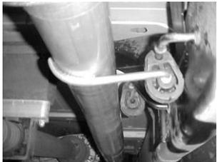
Install down-pipe # A onto intermediate pipe #B 1-1/2"-2". Use clamp # H to secure together, do not tighten. Insert welded hanger into rubber grommet.
