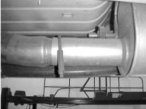
Lay out the exhaust on the floor so it looks like the drawing and compare parts with manual. To remove the stock exhaust remove it from the clamp in front of the muffler. You may need to heat it up for easier removal. Leave all rubber grommets in place. Use WD-40 to aid in removal of exhaust and hangers.
