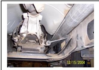
INSTALL TURBO PIPE #A ONTO FACTORY TURBO USING YOUR FACTORY HARDWARE. DO NOT TIGHTEN. INSERT WELDED HANGER INTO RUBBER GROMMET.
