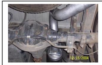
INSTALL OVERAXLE TAILPIPE #E INTO MUFFLER 1-1/2" TO 2". USE CLAMP #J TO SECURE. DO NOT TIGHTEN.
