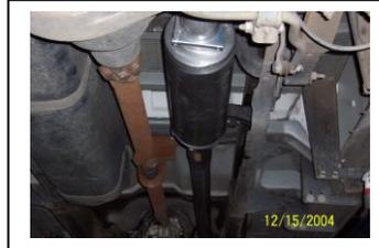
INSTALL REAR MUFFLER HANGER #J ONTO OUTLET OF MUFFLER. INSERT HANGERS INTO RUBBER GROMMETS. DO NOT TIGHTEN.
