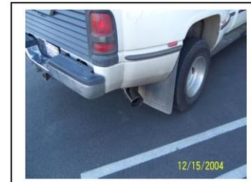
INSTALL YOUR STAINLESS TIP TO YOUR DESIRED LOOK. CHECK FOR CLEARANCES THAN TIGHTEN ALL NUTS, BOLTS AND CLAMPS STARTING FROM THE FRONT AND WORKING YOUR WAY BACK. USE ANY STAINLESS POLISH TO CLEAN TIP.
