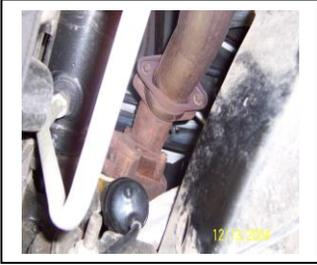
TO INSTALL YOUR DOWNPIPE YOU NEED TO REMOVE YOUR STOCK EXHAUST. TO REMOVE YOUR STOCK EXHAUST UNCLAMP IT JUST IN FRONT OF YOUR STOCK MUFFLER, THEN REMOVE THE REMAINING EXHAUST FROM THE TURBO HOUSING. USE WD-40 TO AID IN REMOVAL OF HANGERS FROM RUBBER GROMMETS. DO NOT DISCARD YOUR STOCK BOLTS FROM YOUR TURBO, YOU WILL RE-USE THEM.
