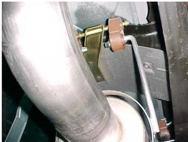
Install band clamp # G into rubber grommets located just above the axle. Do not tighten.
