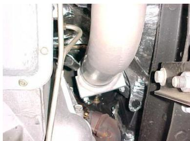
INSTALL DOWN PIPE #K ONTO TURBO USING YOUR FACORY CLAMP. LEAVE LOOSE. DO NOT TIGHTEN .
