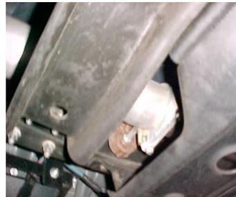
NEXT INSTALL DOWN PIPE HANGERS #N AND #O. INSERT HANGERS INTO RUBBER GROMMETS. DO NOT TIGHTEN.
