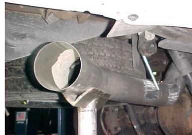
Next Install turnout pipe #D onto tailpipe. Insert welded hanger into rubber grommet. Use clamp #H to secure pipes together. Do not tighten.
