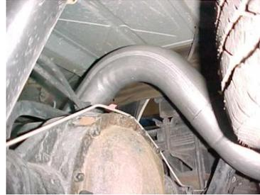
Install the over axle tailpipe # C into the muffler 1-1/2" to 2". Secure to the muffler using clamp # H Do not tighten.
