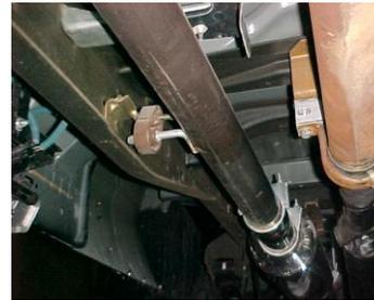
INSTALL THE STRAIGHT PIPE #M ONTO PIPE #L. USE CLAMP #I TO SECURE. DO NOT TIGHTEN.
