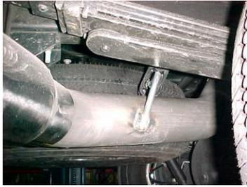
INSTALL THE OVERAXLE TAIL PIPE #D INTO THE MUFFLER 1½"-2", SECURE TO MUFFLER USING CLAMP #F. INSERT WELDED HANGERS INTO RUBBER GROMMETS. DO NOT TIGHTEN.
