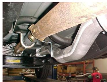
INSTALL DOWN PIPE #B ONTO DOWN PIPE #A. USING GASKET # H AND BOLT KIT # G. INSERT WELDED HANGERS INTO RUBBER GROMMETS. DO NOT TIGHTEN.
